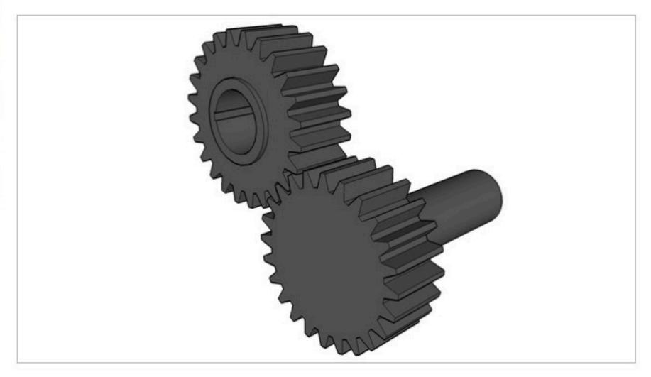
Spur gears are the most common type of gears. They have straight teeth, and are mounted on parallel shafts. Sometimes, many spur gears are used at once to create very large gear reductions.
