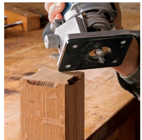
Coves lighten the feet. With the leg post in a vise, using a handheld laminate trimmer (with a ¼-in. bearing-guided cove bit), move in at one pencil mark and out at the other.
