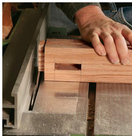
Stub tenons on the tablesaw. The tenon at the top of each leg post is formed with a series of passes on the tablesaw, using the rip fence as a stop and rotating the post.
